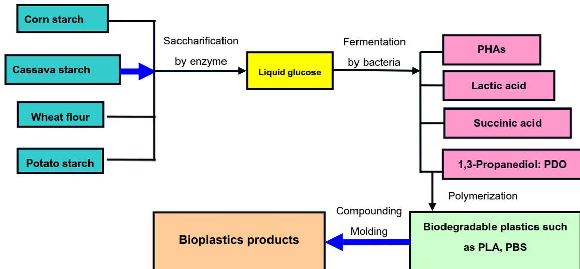
**Figure 1.1** Production process of bioplastics products from biomass
